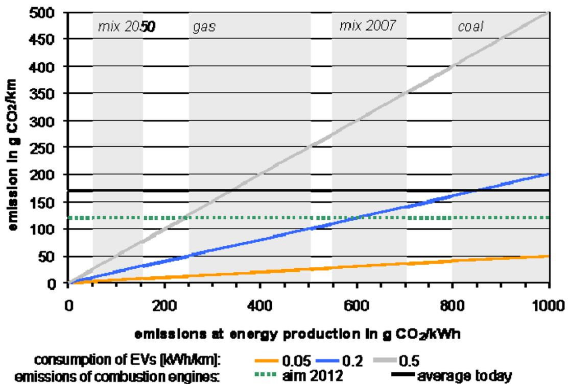
In order to illustrate the connection between CO<sub>2</sub> emissions and sources of electricity generation, figure 1 compares emissions of different BEV pursuant to their consumption as well as average and targeted emissions for new vehicles with combustion engines. The emissions for produced electricity in gram CO<sub>2</sub>
