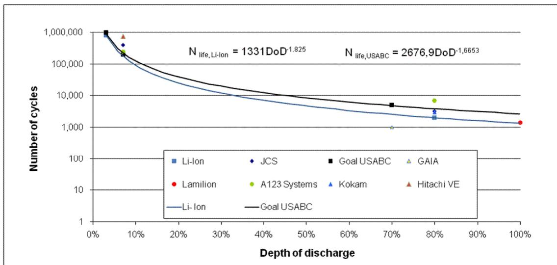
Own calculations based on data in [12] and [13]. For shallow cycles a 7% DoD is used. The battery ageing due to calendar life is not taken into account.
