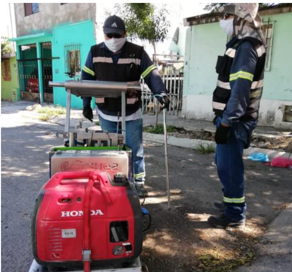
Figure 13: AGSAL workers using iDroloc system for detecting invisible leaks (AGSAL 2019)
