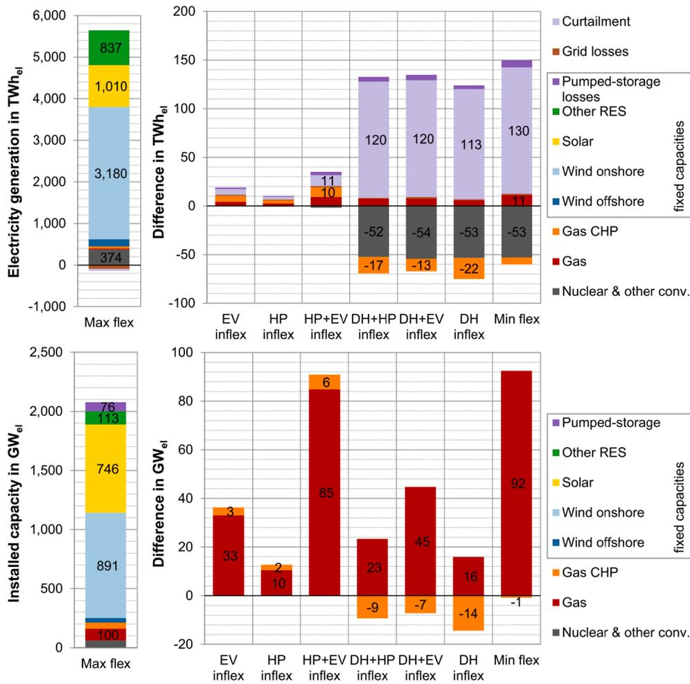
Fig. 5. Electricity generation (top) and installed capacities (bottom) in Europe in 2050 in the *Max flex* scenario and differences of the other scenarios relative to the *Max flex* scenario.
