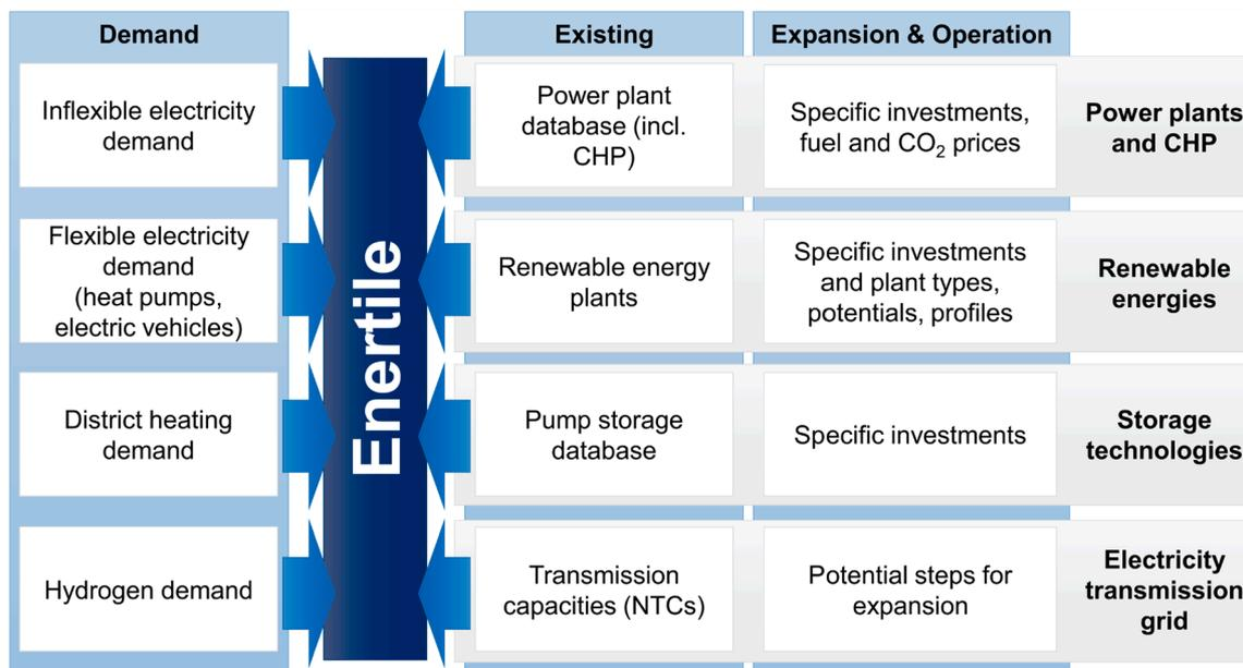
Fig. 1. General structure of the energy system model *EnerTile*.
