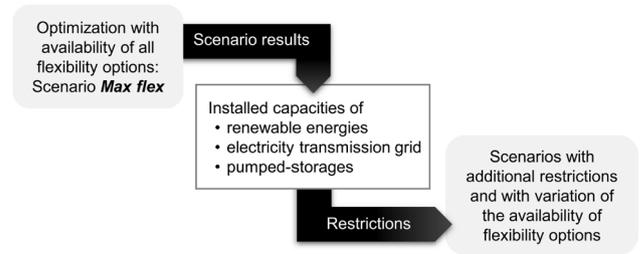
Fig. 3. Procedure for the calculation of the scenarios.
