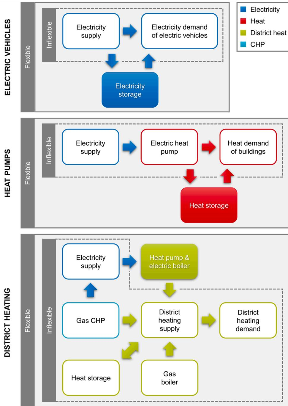
Fig. 2. Modeling the inflexible and flexible operation of electric vehicles, decentralized heat pumps in buildings, and multivalent district heating grids.
