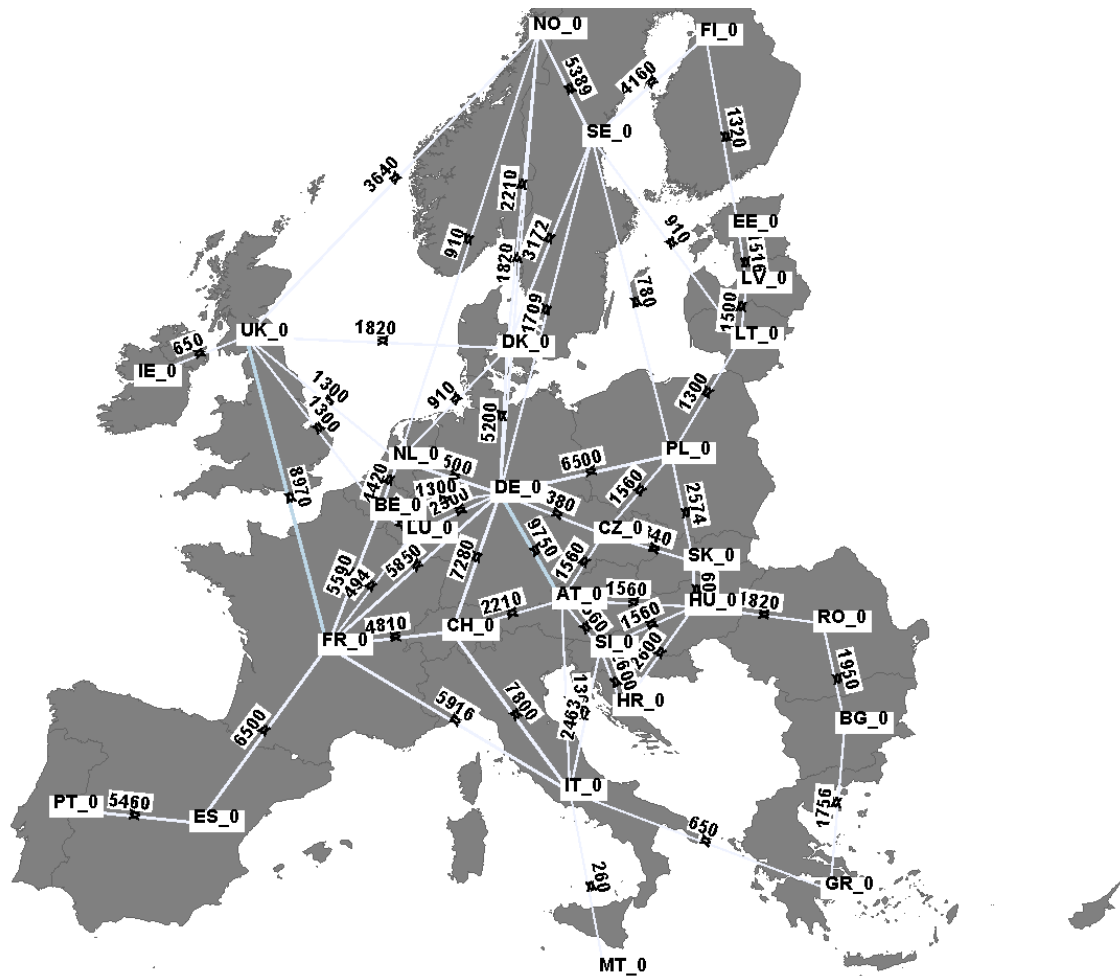
Figure 22: European network of interconnectors with limited grid expansion 10 [in MW]
