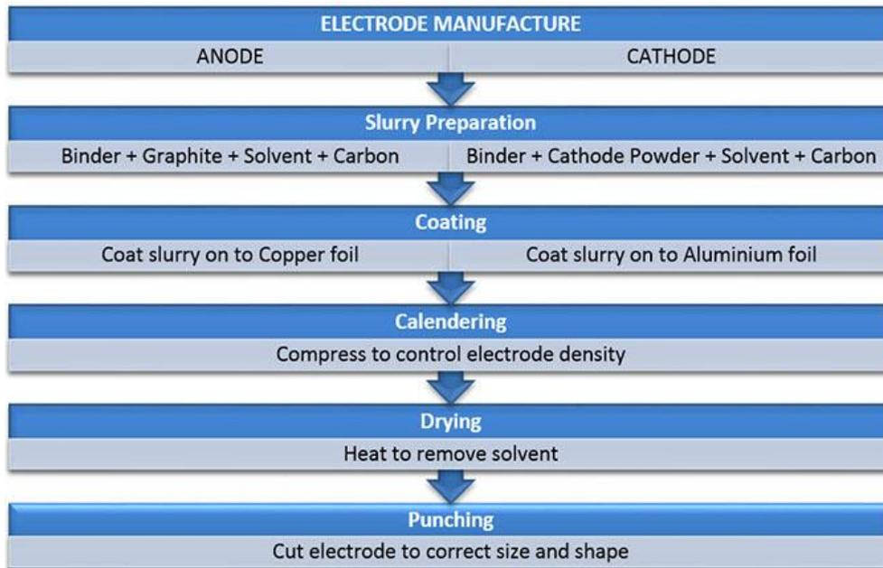
Figure 31: General process of electrode manufacturing for batteries<sup>125</sup>.
