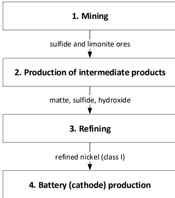
Figure 36: Stylized representation of the nickel supply chain for Li-ion batteries.
