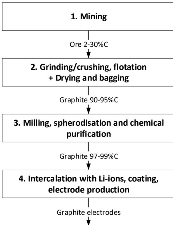
Figure 43: Stylized representation of the natural graphite supply chain for Li-ion batteries<sup>179</sup>.
