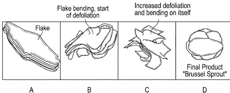
Figure 44: illustration of flake re-shaping transformation process. A: pure graphite flake, B: After substantial impacts with the processing equipment, the flake starts to bend and partially disintegrate at the edges, C: After further processing more substantial defoliation and dislocation of the flake occurs and more substantial bending of these defoliated layers, D: final product, the approximately spherical, rounded particle<sup>192</sup>.
