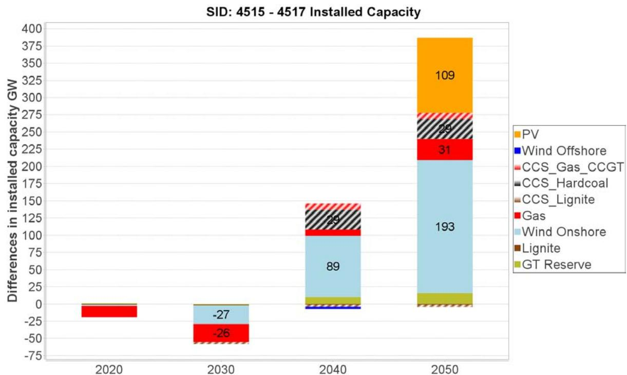
**Figure 19 Impact of higher demand on installed capacity (Scenario D- Scenario C)**
