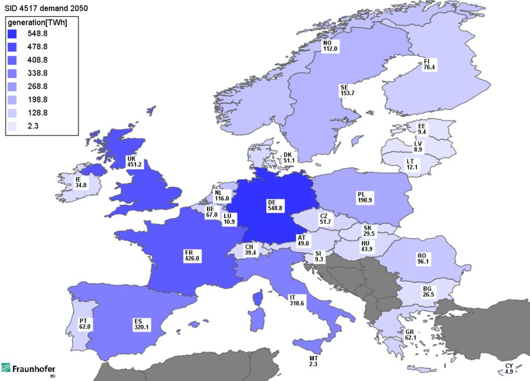
Figure 39 Demand incl. national grid losses in 2050 as assumed in Scenario C and Scenario E
