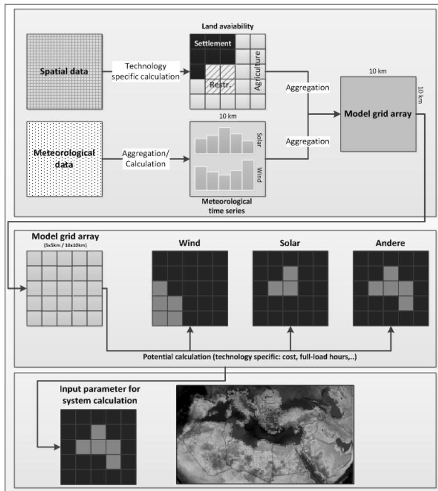
**Figure 10 Model overview of the RE potential calculation**
