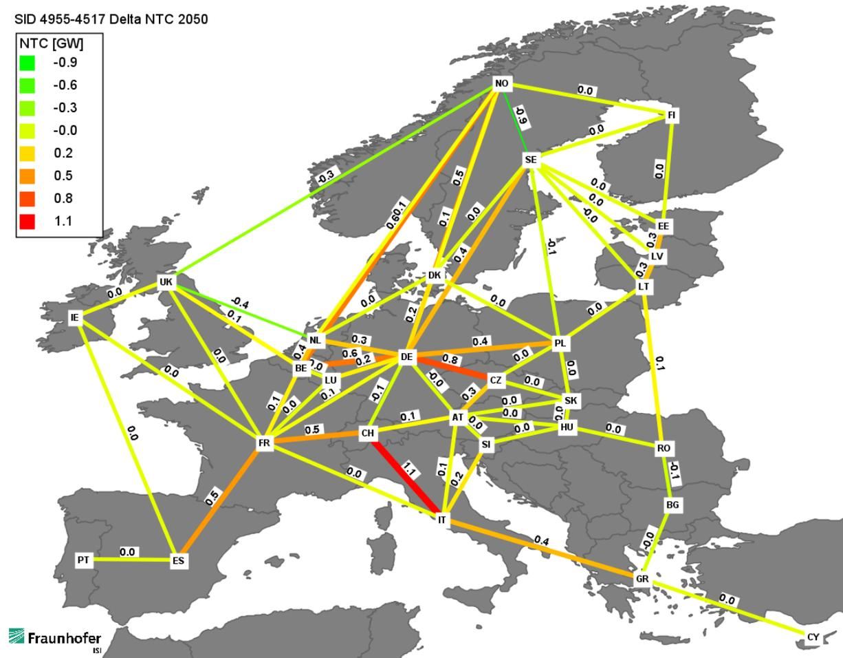
Figure 34 Impact on changed wind assumptions on interconnector capacity (Scenario E- Scenario C) in 2050
