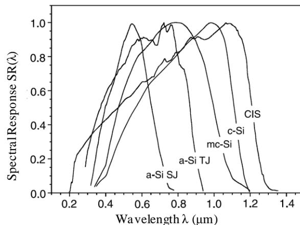
**Figure 1 Spectral Response (SR) for different cell types** (Kenny et al. 2006).
