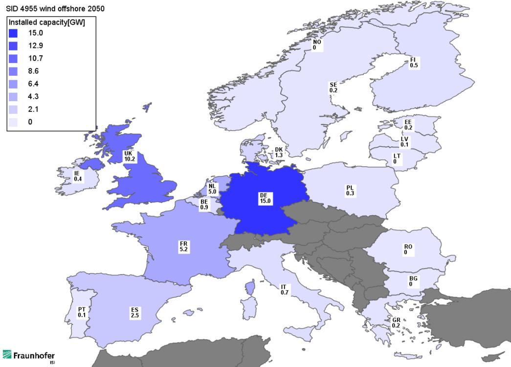
Figure 56 Installed capacity wind offshore Scenario E in 2050
