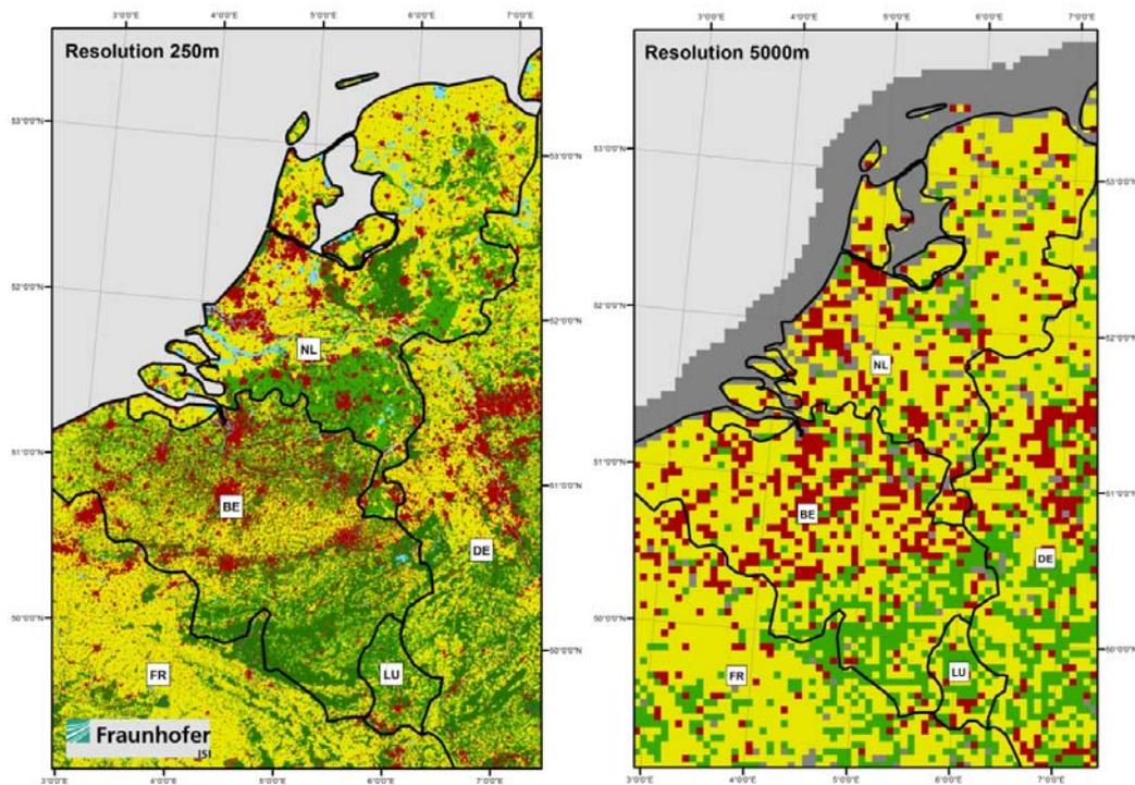
**Figure 59** Example of different land use resolutions based on the CORINE land cover
