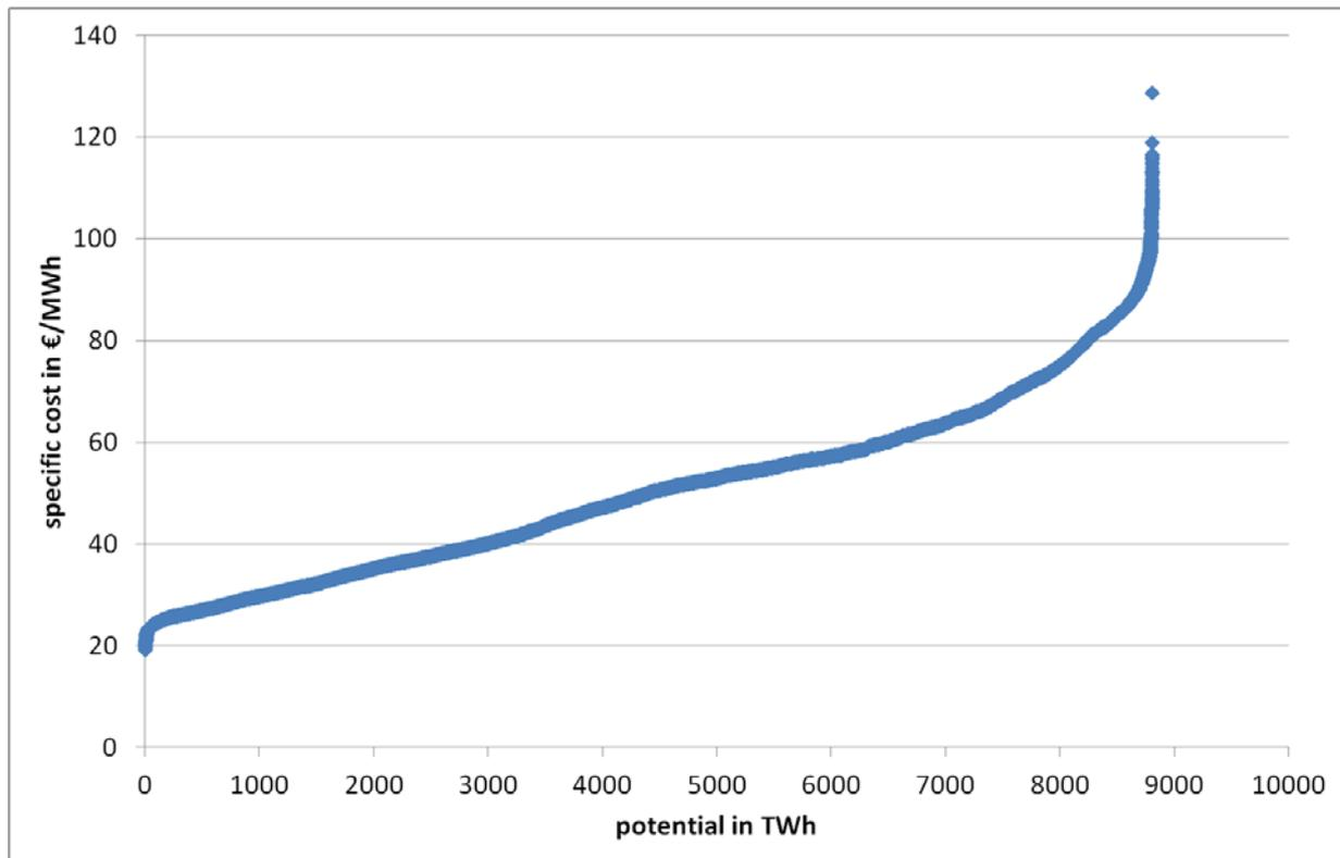
**Figure 13 Generation potential for wind and solar technologies 2050 (here illustrated for Scenario C “Efficiency” and Scenario D (“High Demand”))**
