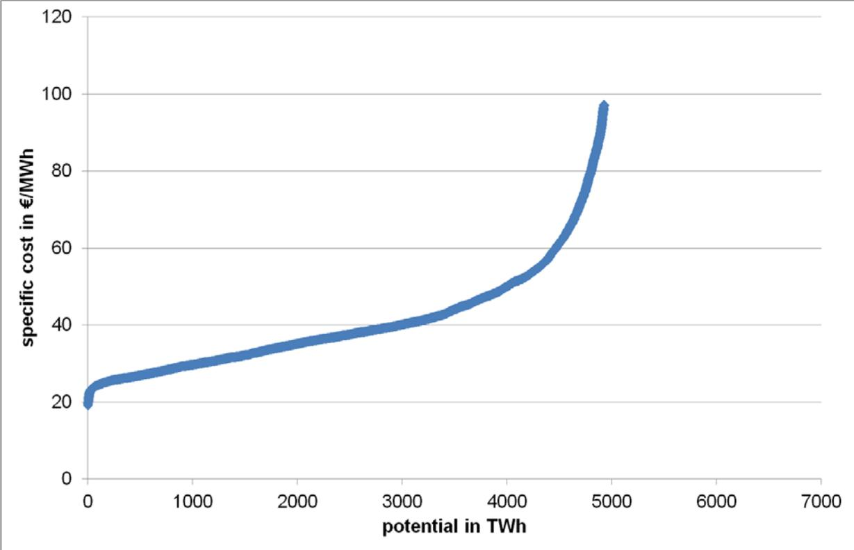
Figure 14 Generation potential for wind onshore in Scenario C ("Efficiency") and Scenario D ("High Demand")
