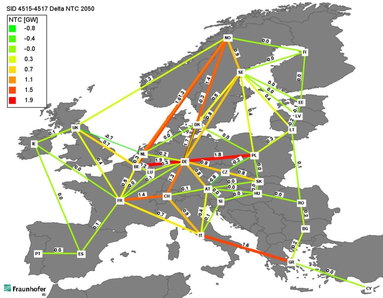
Figure 33 Impact of higher demand on total interconnector capacity (Scenario D- Scenario C) in 2050
