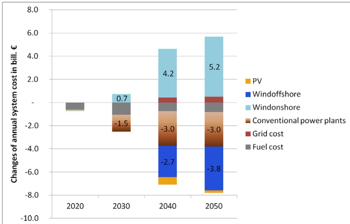
Figure 37 Impact of changed wind assumptions on system cost
