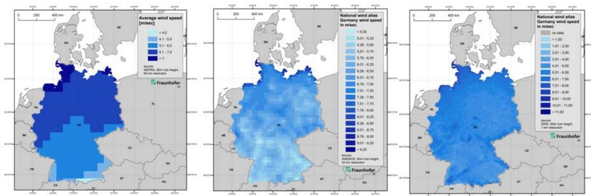
Figure 58 Differences in the wind data resolution
