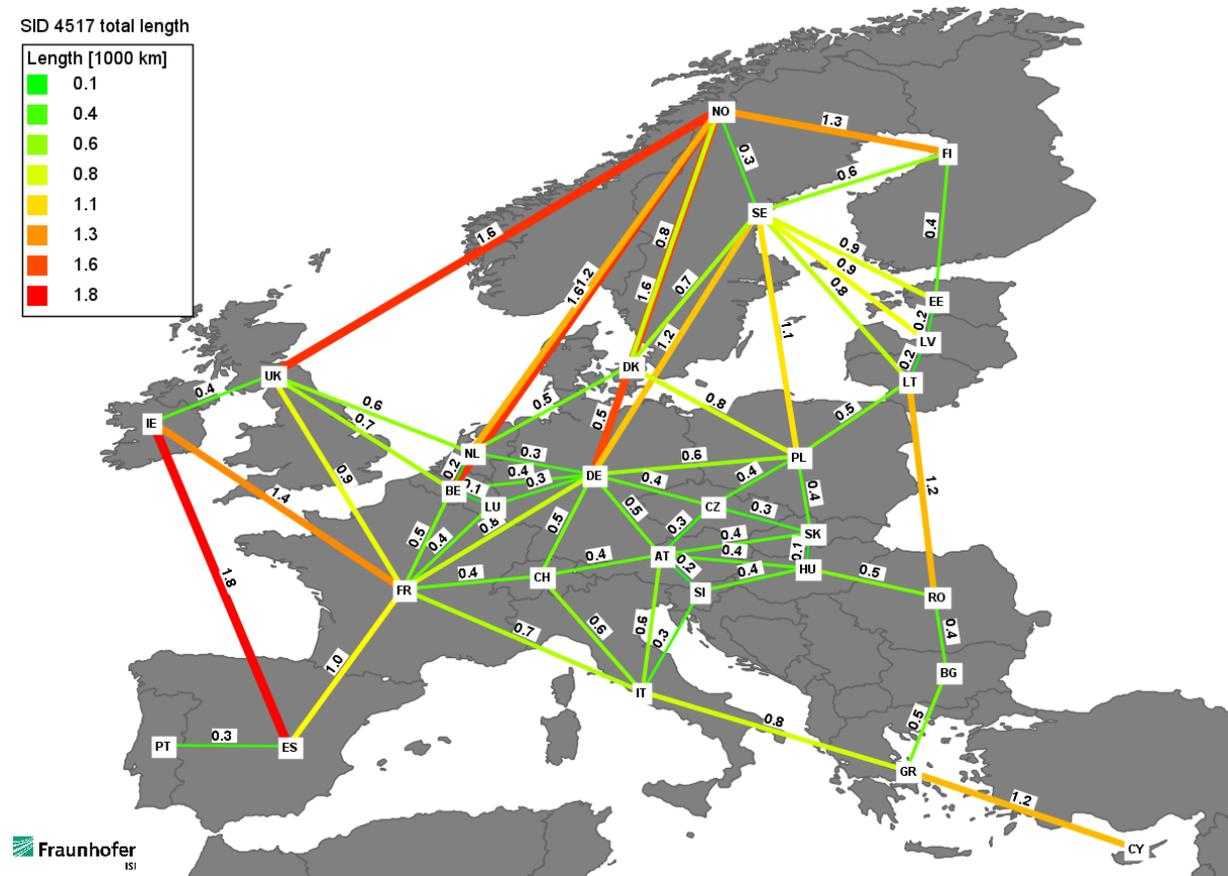
**Figure 6 Transport distances in the underlying grid model**
