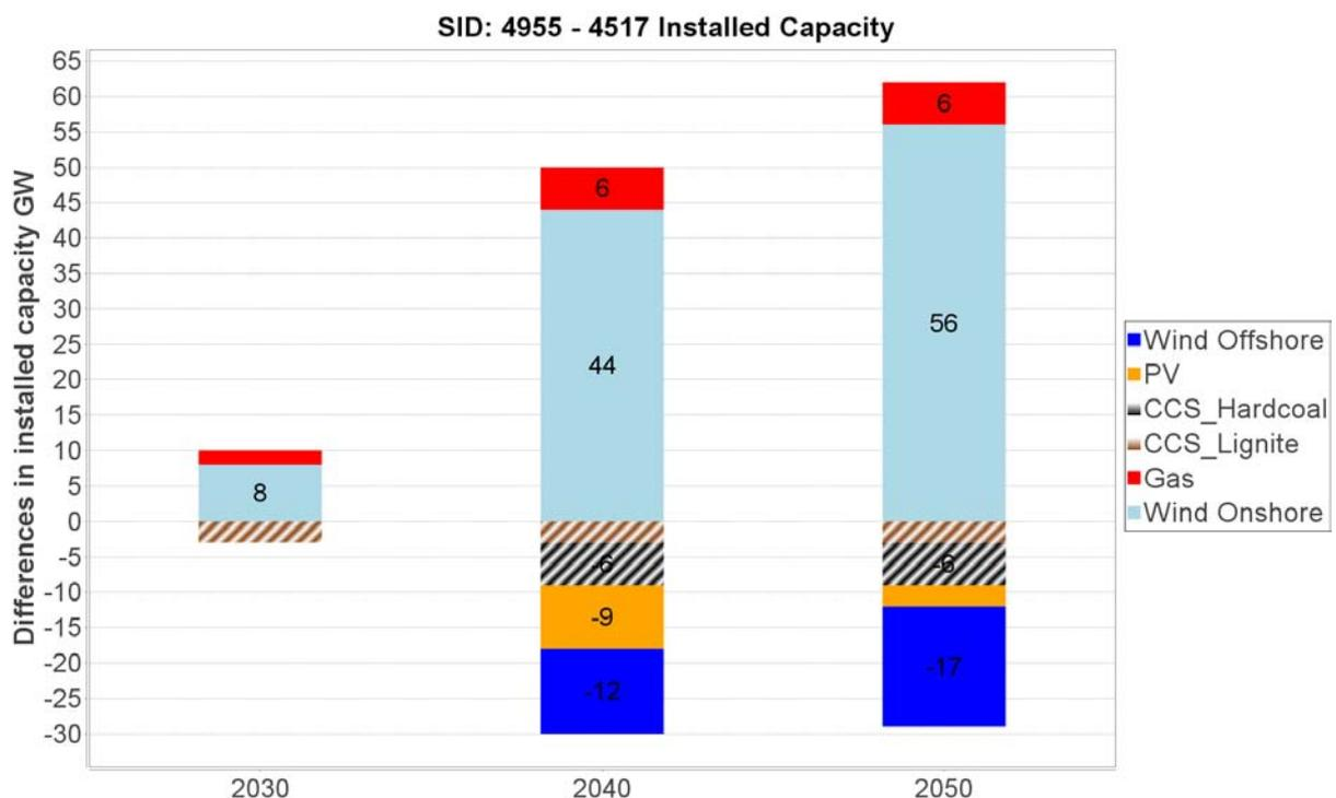
Figure 21 Impact of changed wind assumptions on installed capacity (Scenario E- Scenario C)
