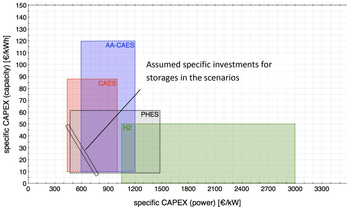
Figure 9 Possible specific investment ranges for 8 hours of storage for pumped hydro electric storage (PHEC), (advanced adiabatic compressed air energy storage [(AA-) CAES] and hydrogen storages (H2)<sup>8</sup>
