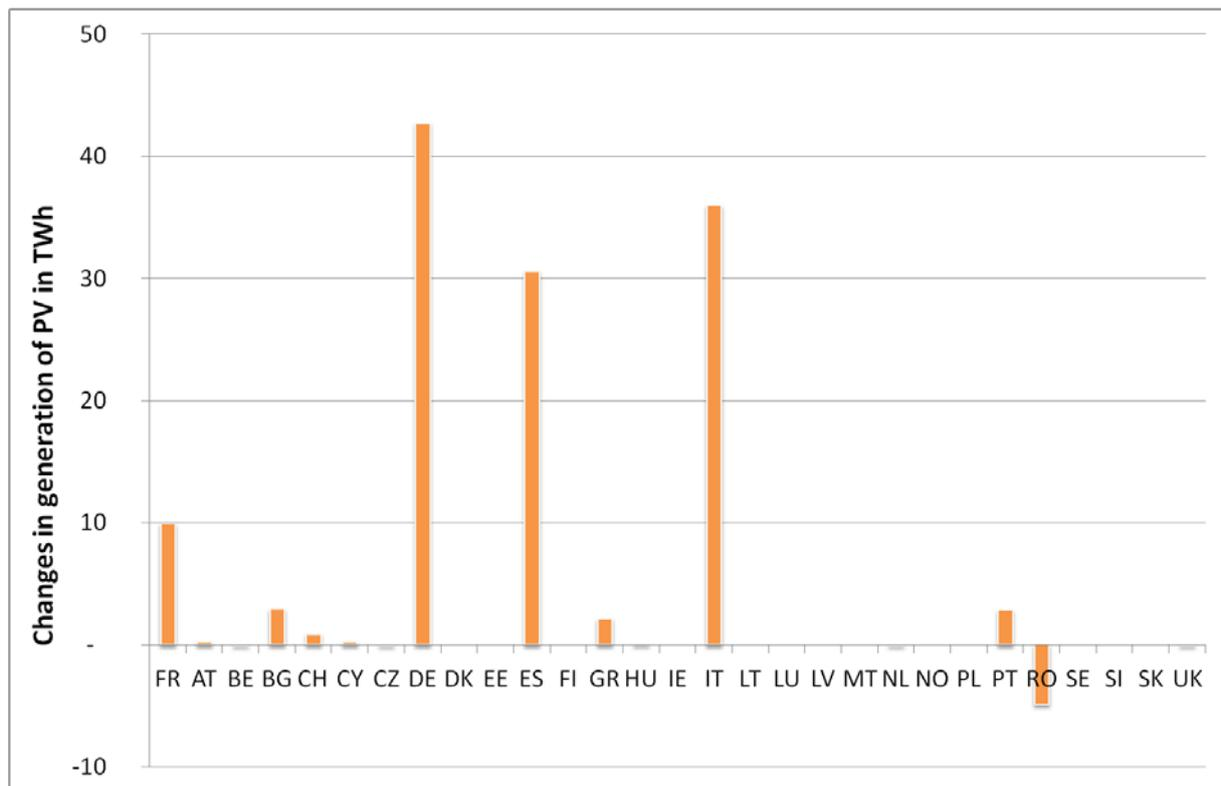
Figure 28 Impact of higher demand on PV generation in 2050 (Scenario D –Scenario C)
