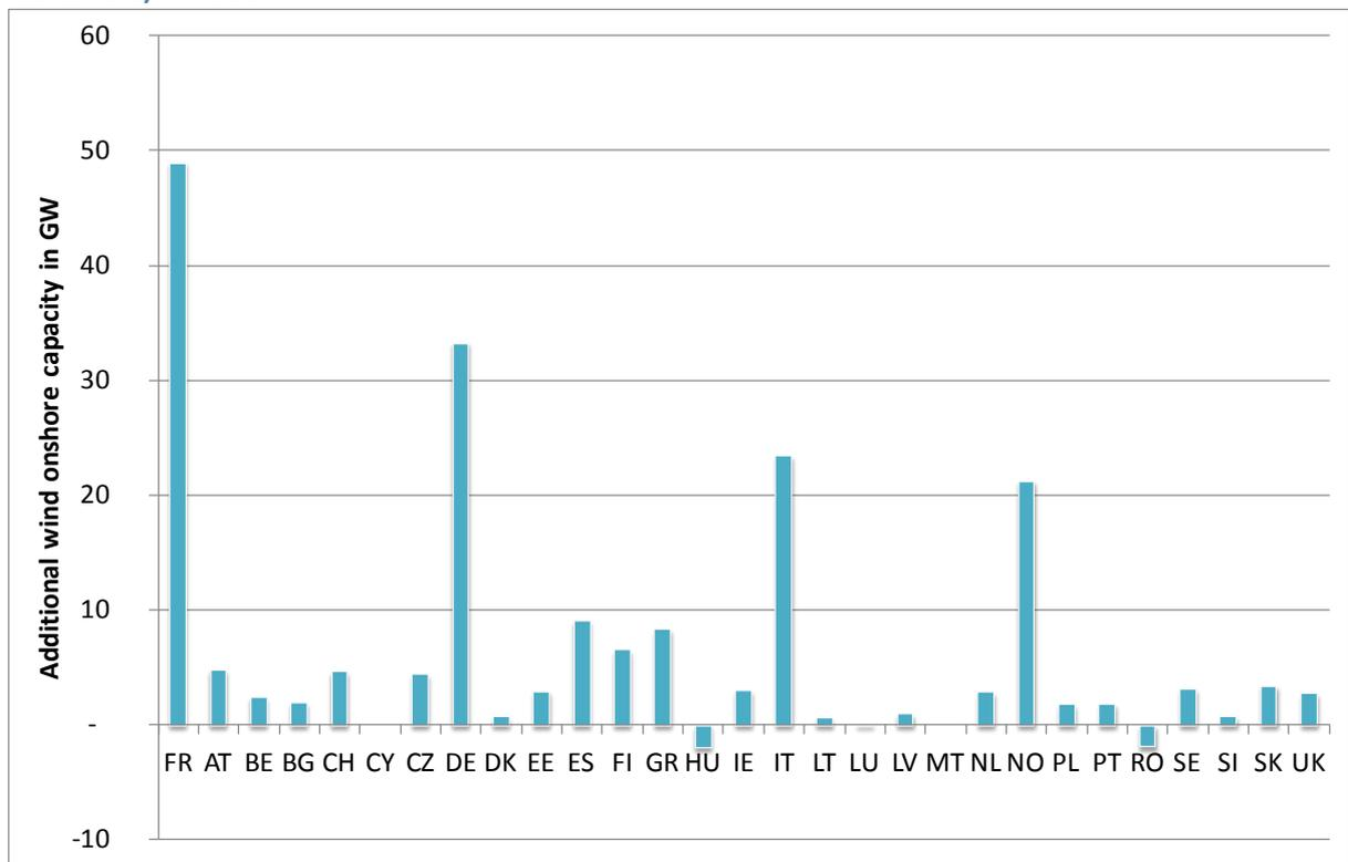
Figure 24 Comparison of additional wind onshore capacity due to higher demand in 2050 (Scenario D – Scenario C)
