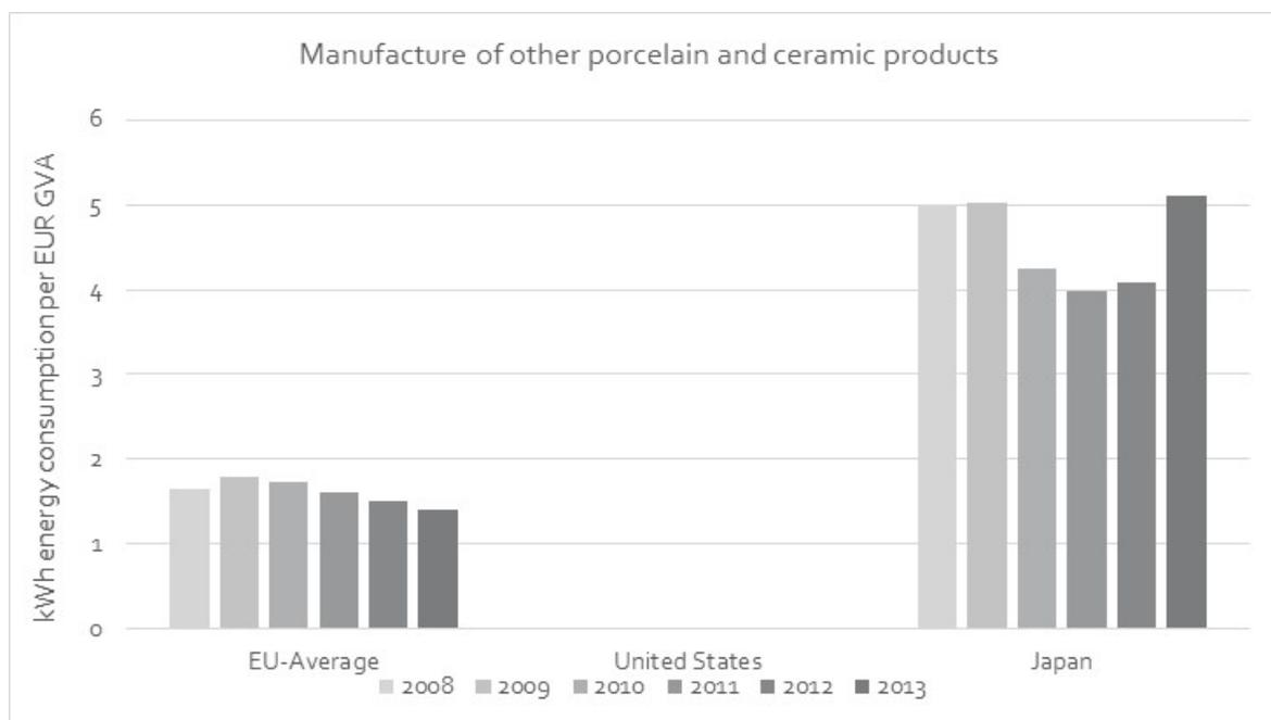
Figure 54 International comparison, energy intensity (energy consumption per EUR GVA generated)
