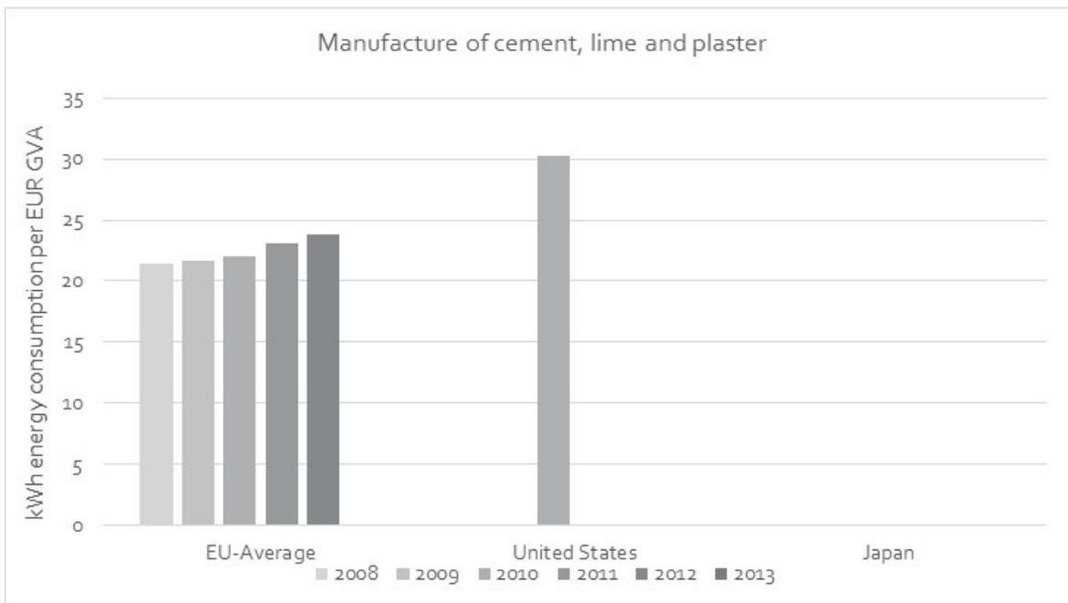
Figure 59 International comparison, energy intensity (energy consumption per EUR GVA generated)
