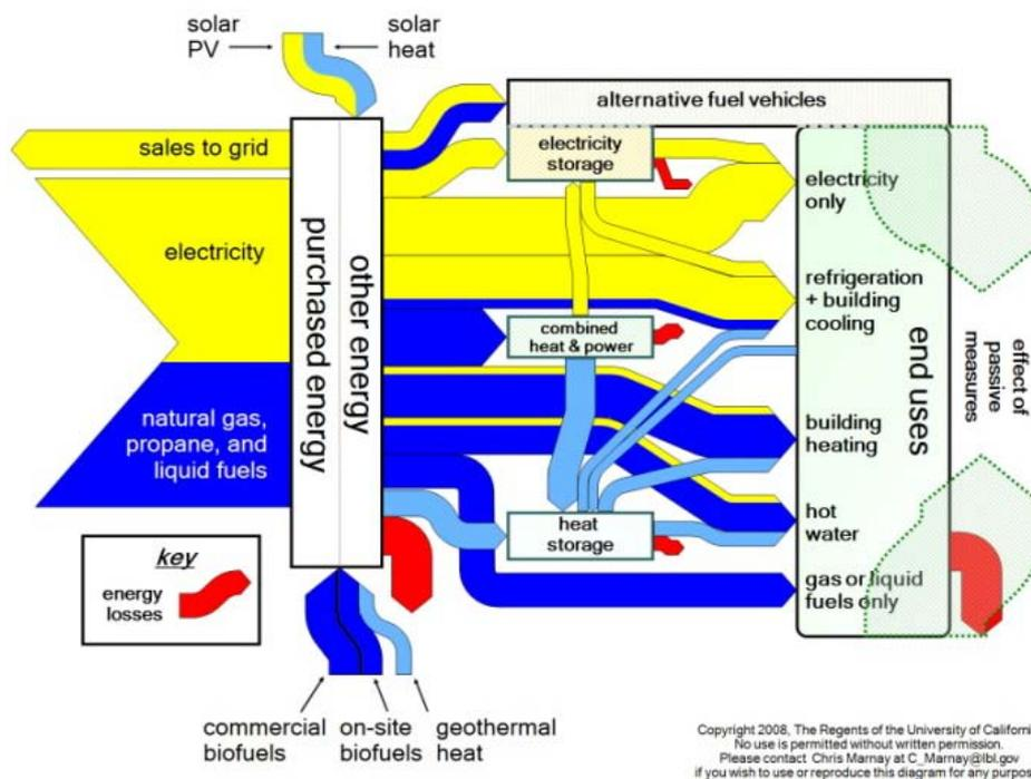
Optimal combinations of equipment involving PV, thermal generation with heat recovery, thermal heat collection, heat-activated cooling, and both thermal and electrical storage can be identified in a way intractable by simple searching. DER-CAM can report a cost, carbon footprint, or combination minimizing equipment choice and (typically hourly) optimal operating schedule for the microgrid/smartgrid, including CHP and renewable sources. The economics of
