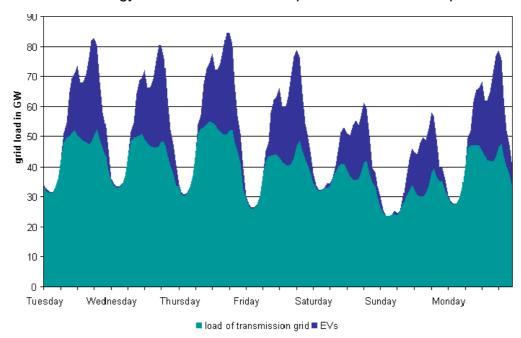
**Assumptions:** 3.5 kWh grid conection; 90% efficiency battery charging; electric vehicles (approx.41.3 Mio.), thereof: BEV: 150 km electr. range and 0.18 kWh energy use per km
