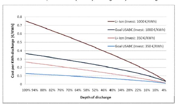
Figure 5: Battery degradation costs for a currently available battery (Li-Ion) and a battery with cycle life given by the USABC goal
