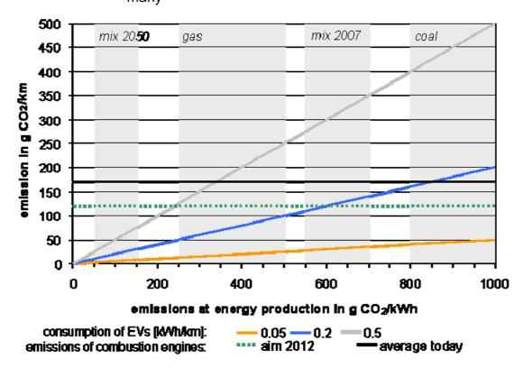
In order to illustrate the connection between CO<sub>2</sub> emissions and sources of electricity generation, figure 1 compares emissions of different BEV pursuant to their consumption as well as average and targeted emissions for new vehicles with combustion engines. The emissions for produced electricity in gram CO<sub>2</sub>
