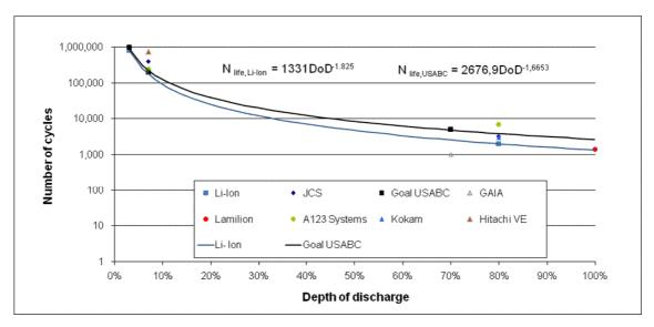
Own calculations based on data in [12] and [13]. For shallow cycles a 7% DoD is used. The battery ageing due to calendar life is not taken into account.
