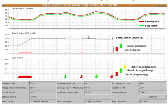
Figure 6: Visualisation and graphical interface of the optimised battery charge dispatch based on the graph search algorithm
