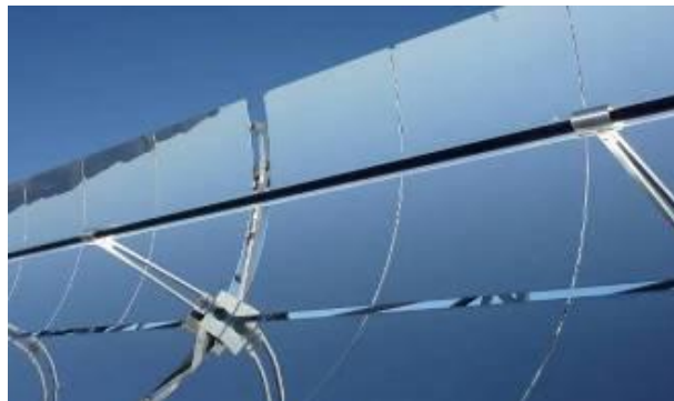
Figure 68: Mirrors in a parabolic trough collector at the Nevada Solar One power plant (source: Morin, 2010)
