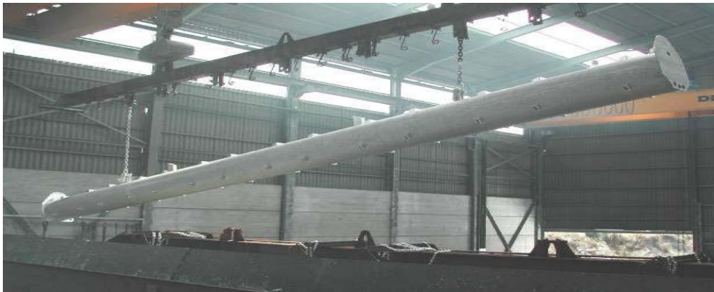
Figure 27 Hot dip galvanizing of a whole torque tube
