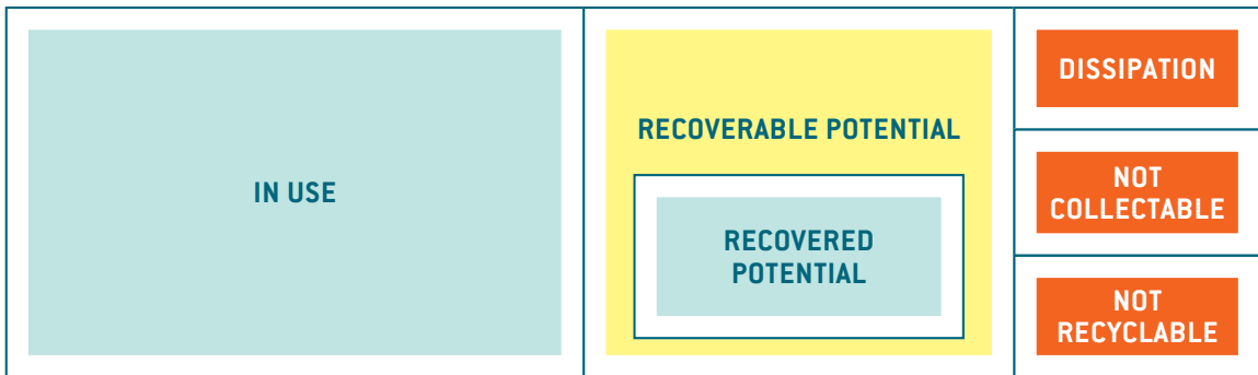
Figure 8: Breakdown of the theoretical potential of the Urban Mine. Products in use are currently not available for recycling. Materials are lost to the environment through dissipation (e.g., corrosion or abrasion) and are not available for recycling. Practical issues such as accessing the scrap (e.g., subterranean cables) or the presence of hazardous chemicals in products/scrap block collection and/or recycling.
